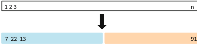
FIGURE 5.1. A schematic display of the validation set approach. A set of n observations are randomly split into a training set (shown in blue, containing observations 7, 22, and 13, among others) and a validation set (shown in beige, and containing observation 91, among others). The statistical learning method is fit on the training set, and its performance is evaluated on the validation set.
